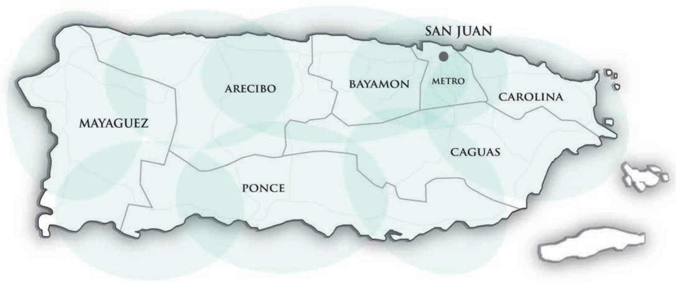
Puerto Rico's microgrid network will feature eight subgrids, powered by smaller generators.
